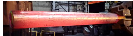
Fig.9 - Appearance of round bar (All forging processes use FDFD)
